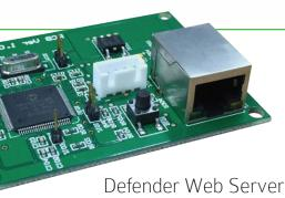
Attach the web server to enable network connectivity, access and control over the network or internet, compatible with Windows and Mac OS.
